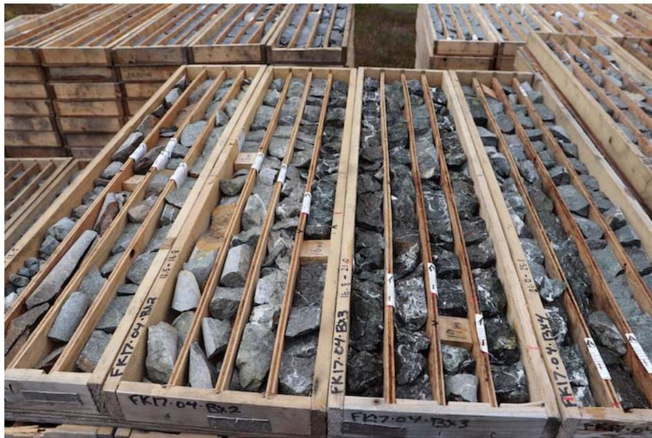
2017 core samples. Hole FK17-04 hit near-surface mineralization 18 to 21m deep, returning grades of 18.9 g/t gold, 16.6 g/t silver, and 2.2% copper
