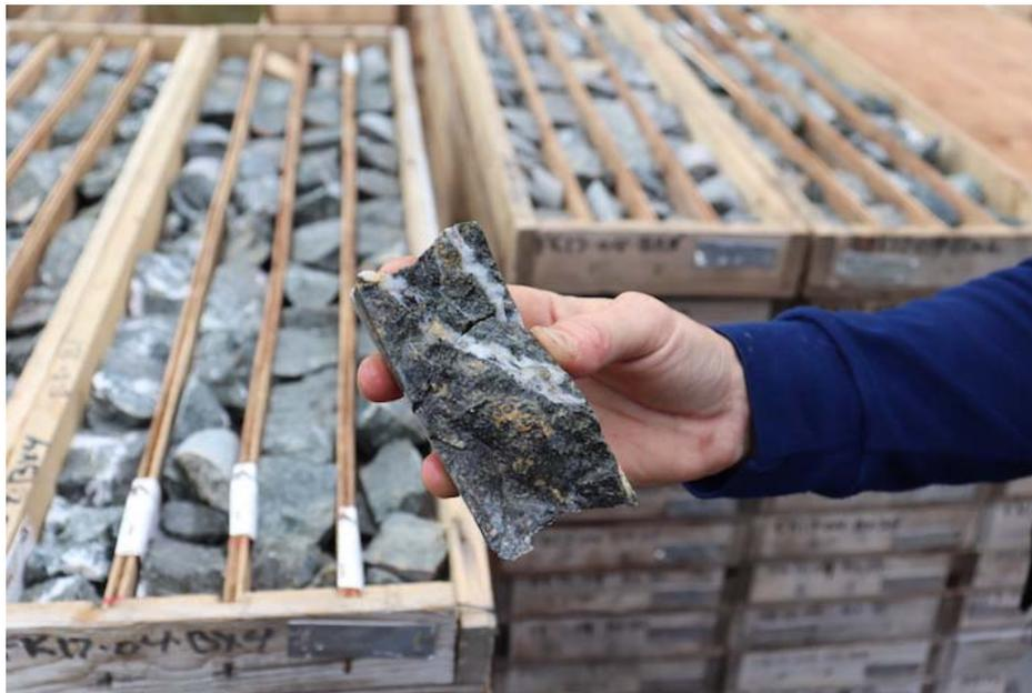
A chunk of mineralized core showing quartz veining and chalcopyrite
